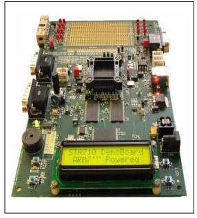
The STR710-EVAL integrates a 2x16 LCD, LEDs, UART, CAN and USB interfaces, piezo buzzer and test buttons in a versatile stand-alone test platform.
