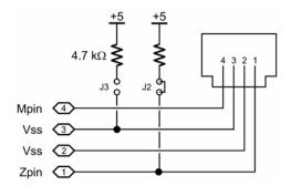
For 1-Wire I/O using a Blue Dot Receptor, configure the RJ-11 port as follows (J3 in, J2 out):
