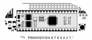
The BS2p40 module can be programmed via the USB port or through a standard serial port.
