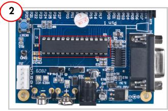
Plug the PSoC CY8C29466 chip into the socket (U2).
