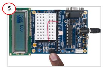
Vary the potentiometer and see the output hex values on the LCD module.
