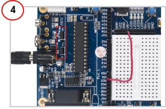
Connect jumper at JP1 and JP2. Connect jumper wire between PO1 and VR.
