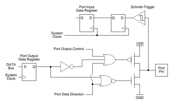
Figure 9. GPIO Port Pin Block Diagram
