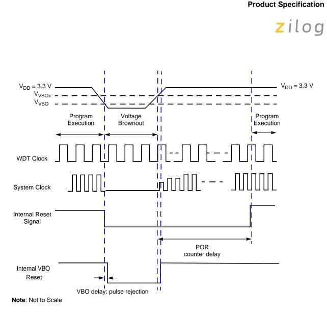
Figure 8. Voltage Brownout Reset Operation
