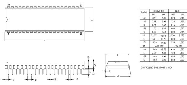
Figure 86. 40-Lead Plastic Dual-Inline Package (PDIP)
