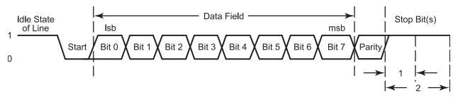
Figure 21. LIN-UART Asynchronous Data Format with Parity
