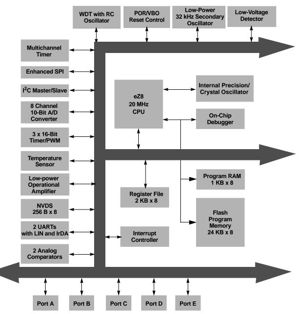
Figure 1. Z8 Encore! XP F1680 Series Block Diagram
