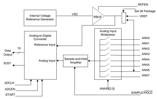
Figure 30. Analog-to-Digital Converter Block Diagram
