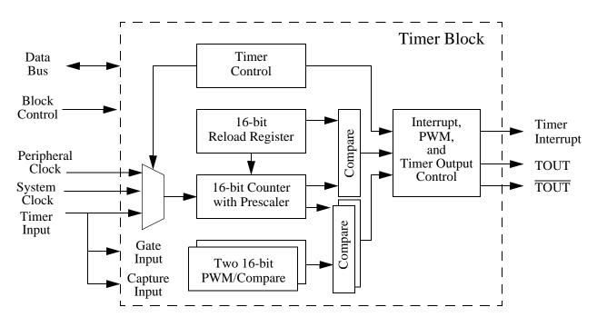
Figure 11. Timer Block Diagram
