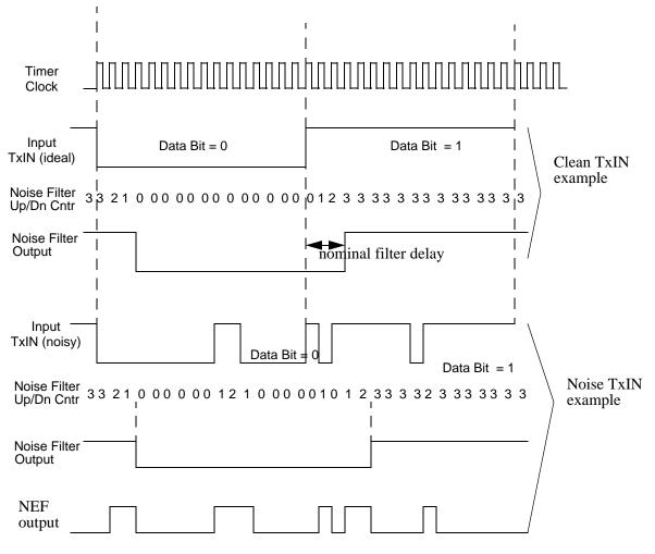
Figure 13. Noise Filter Operation
