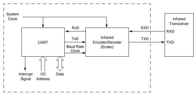
Figure 27 displays the architecture of the Infrared Endec.
