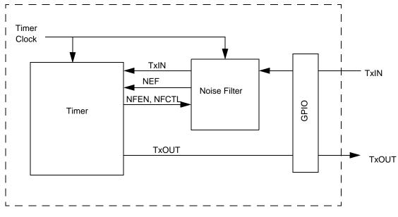
Figure 12. Noise Filter System Block Diagram
