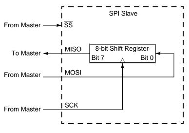
Figure 41. ESPI Configured as an SPI Slave
