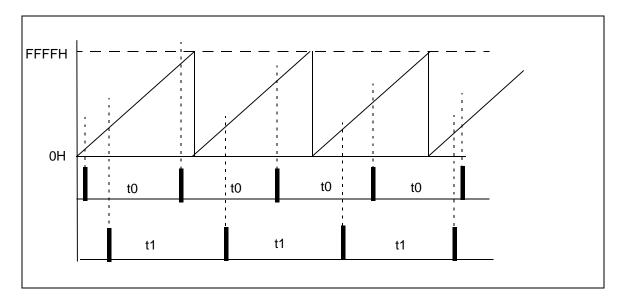
Figure 18. Count Max Mode with Channel Compare
