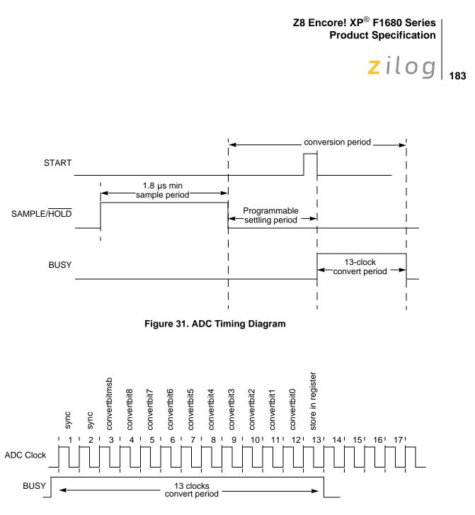
Figure 32. ADC Convert Timing
