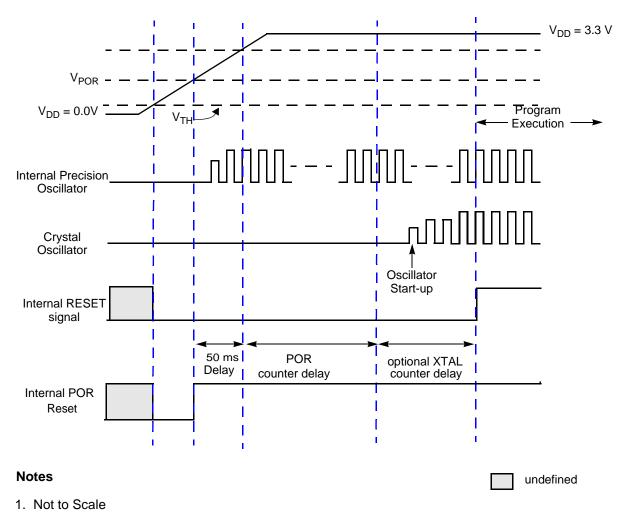
2. Internal Reset and POR Reset are low active
