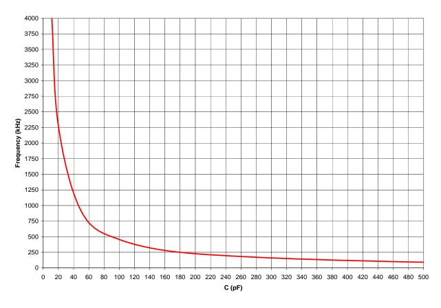
Figure 64. Typical RC Oscillator Frequency as a Function of the External Capacitance with a 45 K $\Omega$  Resistor
