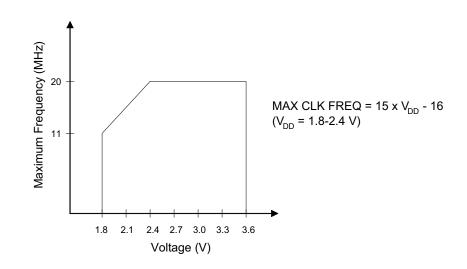
Figure 74. V<sub>DD</sub> Versus Maximum System Clock Frequency
