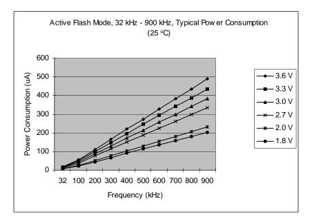
Figure 71. Typical Active Flash Mode Supply Current (32–900 kHz)
