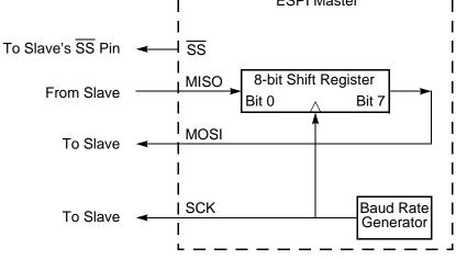
Figure 39. ESPI Configured as an SPI Master in a Single Master, Single Slave System
