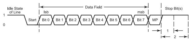
Figure 23. LIN-UART Asynchronous MULTIPROCESSOR Mode Data Format
