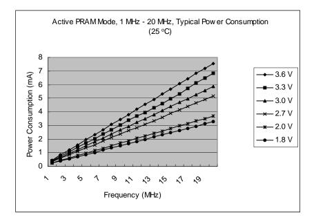
Figure 70. Typical Active PRAM Mode Supply Current (1–20 MHz)
