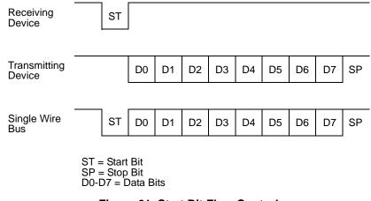
Figure 61. Start Bit Flow Control
