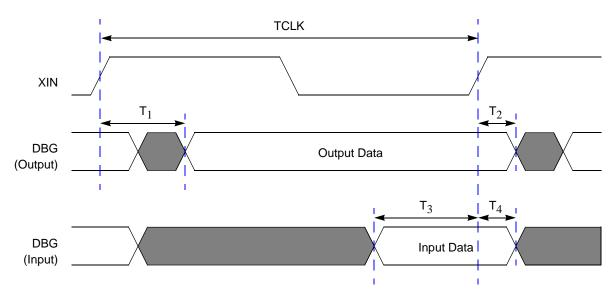
Figure 77. On-Chip Debugger Timing
