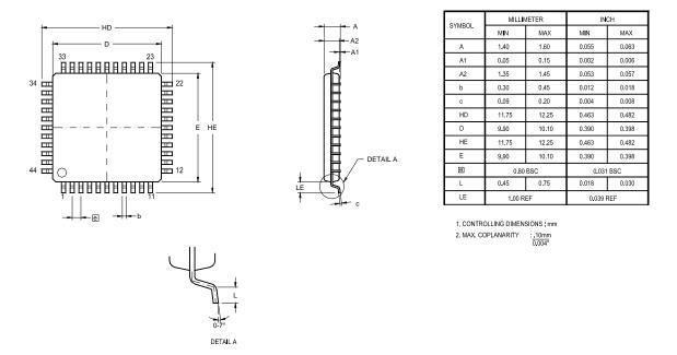
Figure 87 displays the 44-pin Low-Profile Quad Flat Package (LQFP) available for the Z8 Encore! XP F1680 Series devices.
