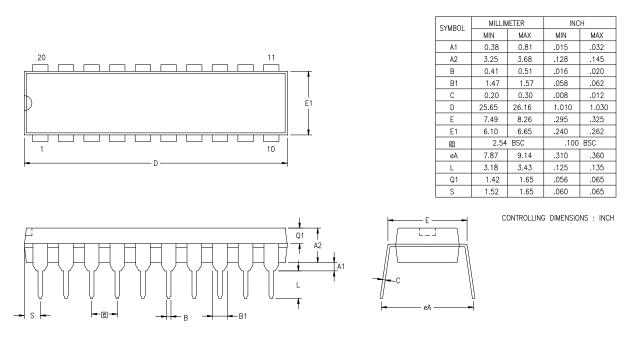
Figure 80. 20-Pin Plastic Dual Inline Package (PDIP)
