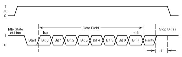
Figure 22. LIN-UART Driver Enable Signal Timing with One Stop Bit and Parity
