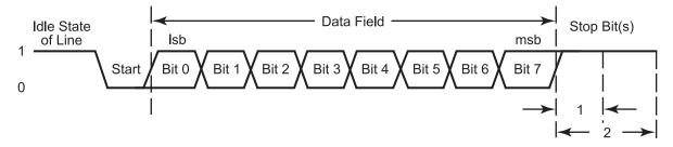
Figure 20. LIN-UART Asynchronous Data Format without Parity
