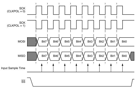
Figure 35. ESPI Timing when PHASE = 1
