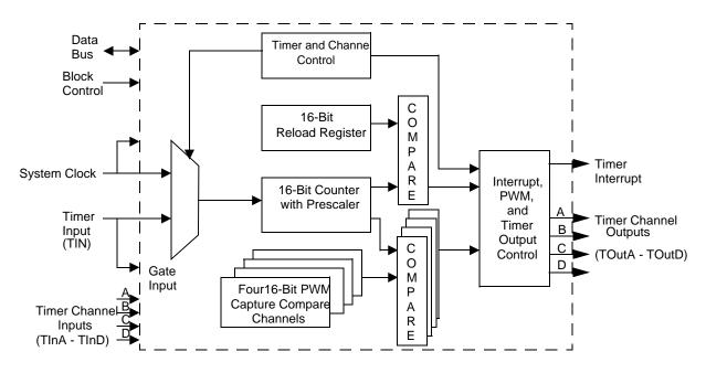
Figure 14. Multi-Channel Timer Block Diagram
