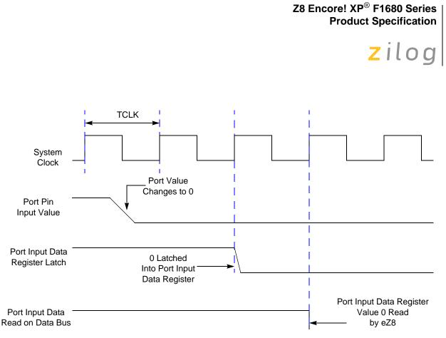
Figure 75. Port Input Sample Timing
