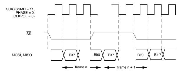
Figure 38. Synchronous Message Framing Mode (SSMD = 11), Multiple Frames
