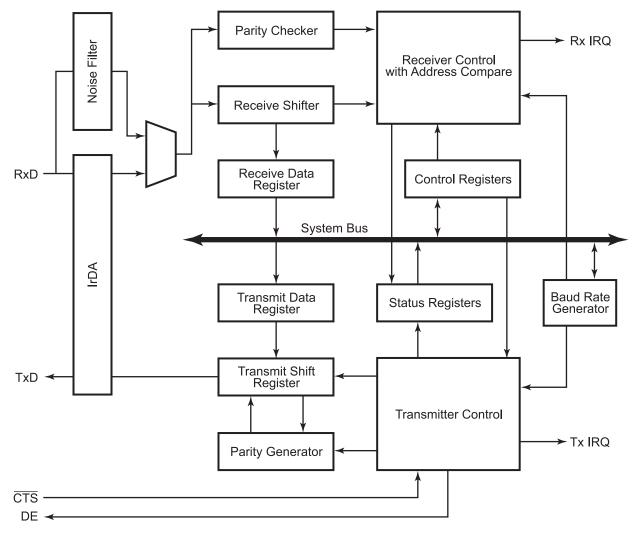
Figure 19. LIN-UART Block Diagram
