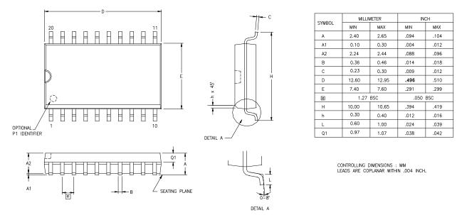
Figure 81. 20-Pin Small Outline Integrated Circuit Package (SOIC)
