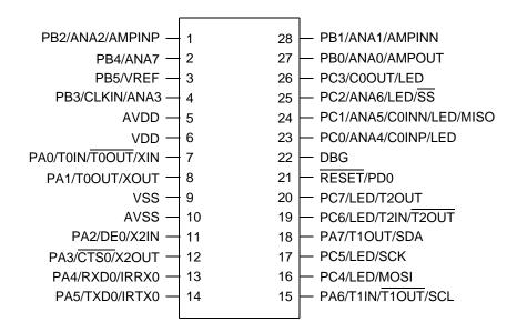
Figure 3. Z8F2480, Z8F1680 and Z8F0880 in 28-Pin SOIC, SSOP or PDIP Packages
