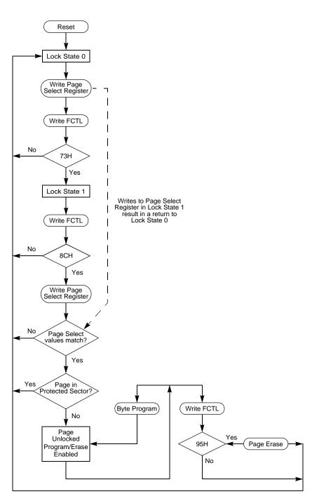
Figure 54. Flash Controller Operation Flowchart
