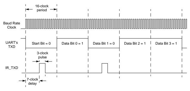
Figure 28. Infrared Data Transmission
