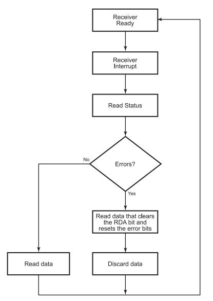
Figure 24. LIN-UART Receiver Interrupt Service Routine Flow
