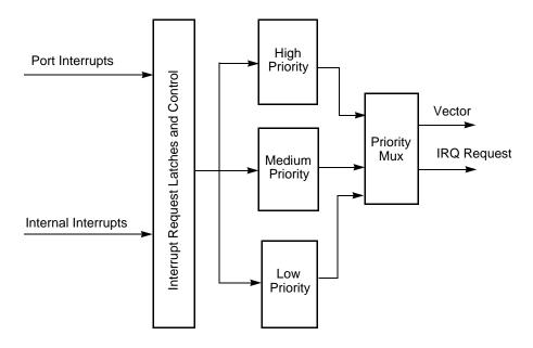
Figure 10. Interrupt Controller Block Diagram
