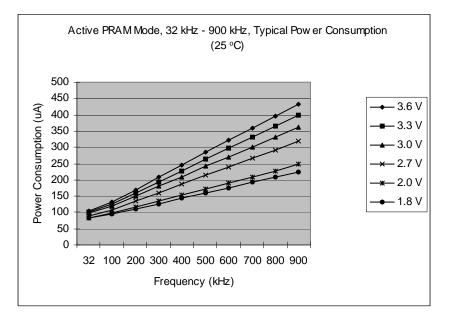
Figure 72. Typical Active PRAM Mode Supply Current (32–900 kHz)
