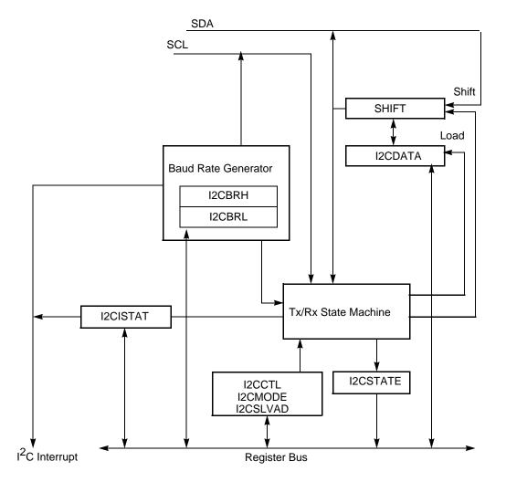
Figure 42. I<sup>2</sup>C Controller Block Diagram
