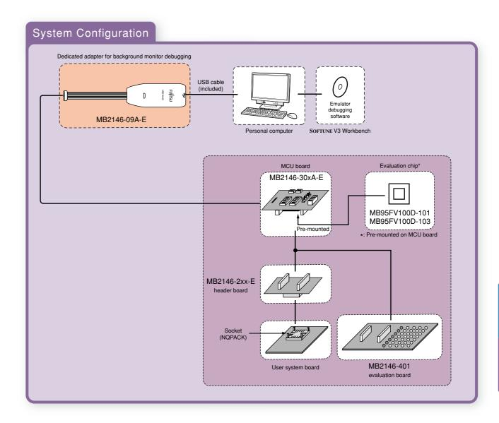
Fujitsu Semiconductor provides ICE, evaluation boards, monitor debuggers, ROM writers, etc. for developing software for the FR family and F<sup>2</sup>MC family.
