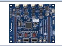
Learning CAN/LIN communication with a particular aim is also possible by combining with a bits pot white (CAN-LIN), bits pot red (CAN-Motor), or bits pot yellow (LIN), and sample programs are also available depending on the combination.
