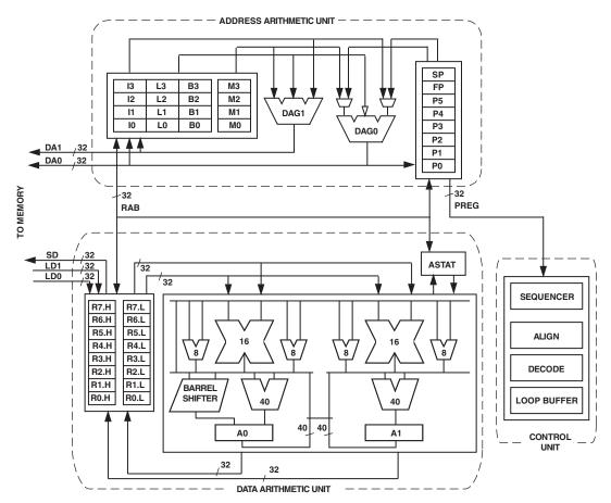
Figure 1. Blackfin Processor Core
