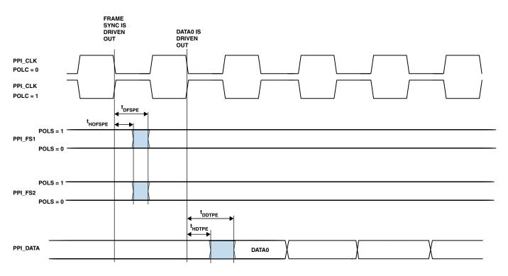
Figure 15. PPI GP Tx Mode with Internal Frame Sync Timing
