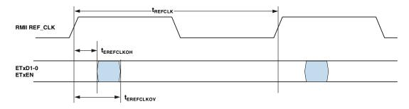
Figure 29. 10/100 Ethernet MAC Controller Timing: RMII Transmit Signal
