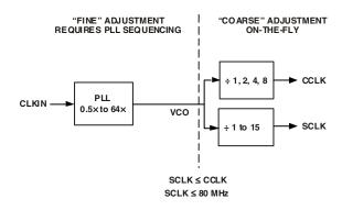
Figure 5. Frequency Modification Methods
