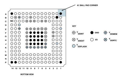
Figure 57. 168-Ball CSP\_BGA Ball Configuration (Bottom View)
