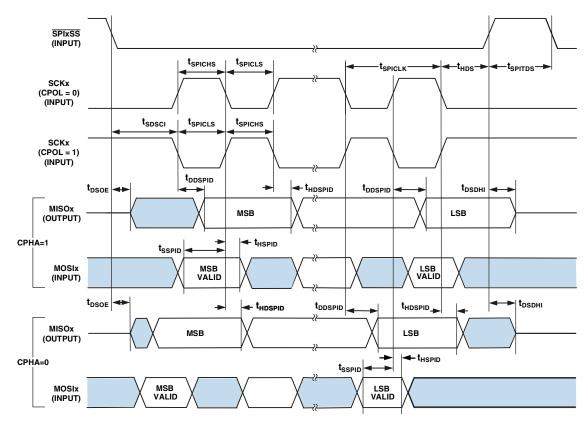
Figure 21. Serial Peripheral Interface (SPI) Port—Slave Timing
