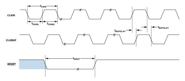
Figure 7. Clock and Reset Timing
