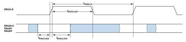
Figure 26. 10/100 Ethernet MAC Controller Timing: MII Receive Signal
