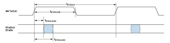
Figure 27. 10/100 Ethernet MAC Controller Timing: MII Transmit Signal
