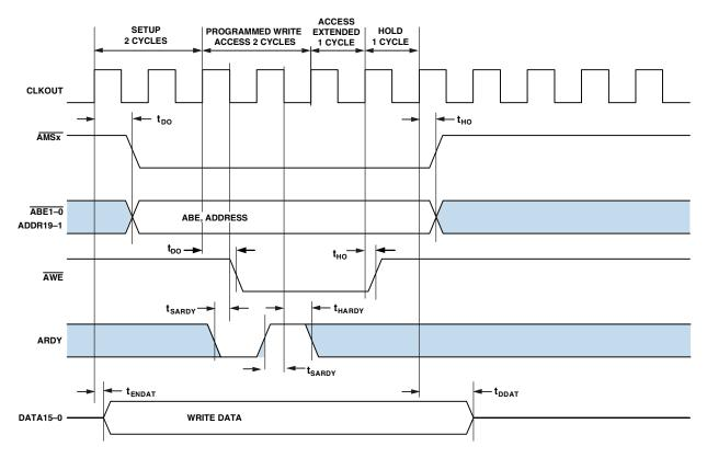
Figure 9. Asynchronous Memory Write Cycle Timing
