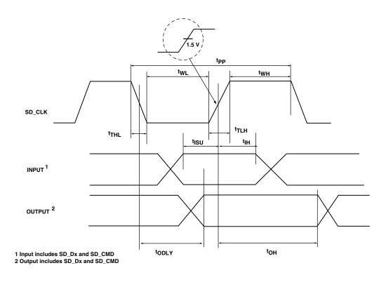
Figure 17. SD/SDIO Controller Timing (High-Speed Mode)
