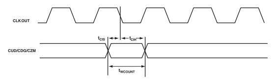
Figure 25. Up/Down Counter/Rotary Encoder Timing
