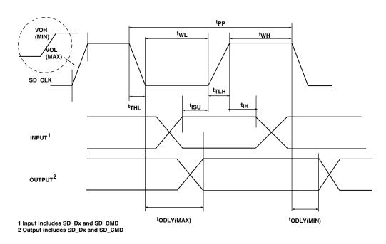
Figure 16. SD/SDIO Controller Timing
