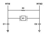
SUGGESTED COMPONENTS: X1 = ECLIPTEK EC38J (THROUGH-HOLE PACKAGE) OR EPSON MC405 12 pF LOAD (SURFACE-MOUNT PACKAGE)
