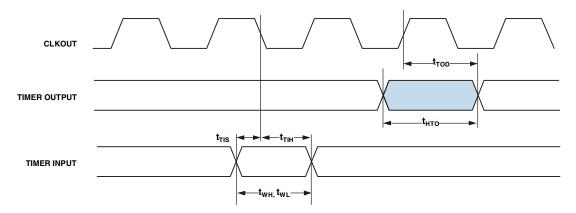
Figure 24. Timer Cycle Timing
