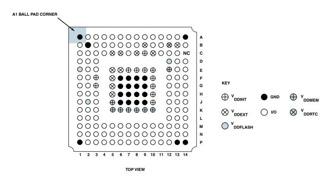
Figure 56. 168-Ball CSP\_BGA Ball Configuration (Top View)
