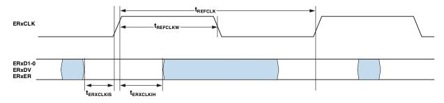
Figure 28. 10/100 Ethernet MAC Controller Timing: RMII Receive Signal
