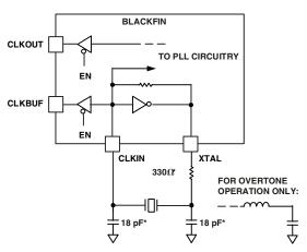
NOTE: VALUES MARKED WITH \* MUST BE CUSTOMIZED DEPENDING ON THE CRYSTAL AND LAYOUT. PLEASE ANALYZE CAREFULLY.
