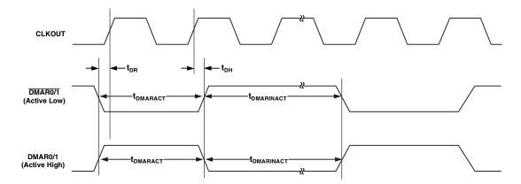
Figure 11. External DMA Request Timing
