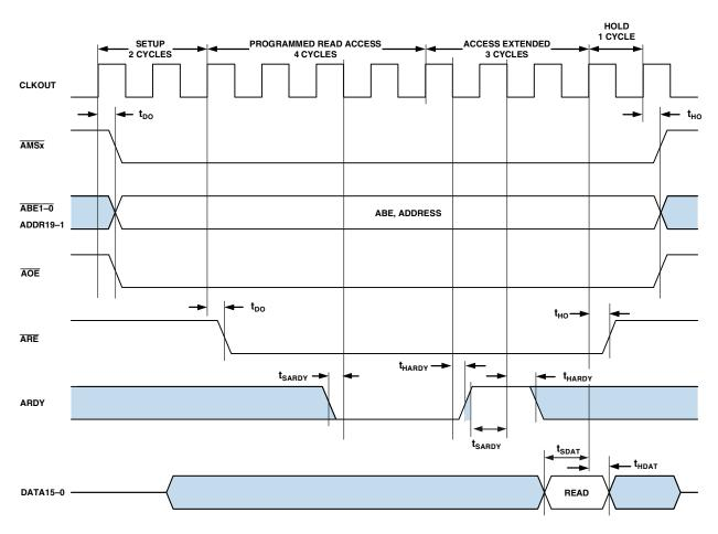
Figure 8. Asynchronous Memory Read Cycle Timing
