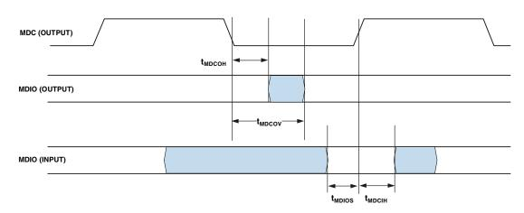
Figure 31. 10/100 Ethernet MAC Controller Timing: MII Station Management
