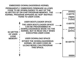
Figure 19. Flash/EE Program Memory Map in ULOAD Mode
