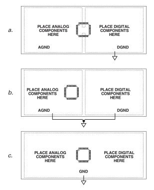
Figure 63. System Grounding Schemes
