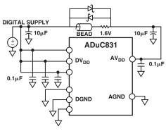
Figure 61. External Single-Supply Connections
