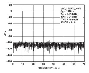
TPC 11. Dynamic Performance at  $V_{DD} = 5 \text{ V}$
