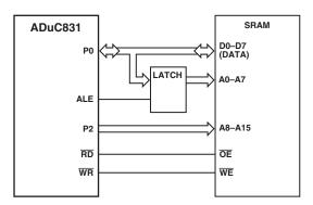
Figure 58. External Data Memory Interface (64 K Address Space)
