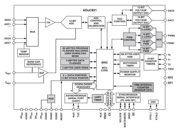
Figure 1. ADuC831 Block Diagram (Shaded areas are features not present on the ADuC812)
