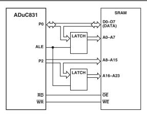
Figure 59. External Data Memory Interface (16 MBytes Address Space)
