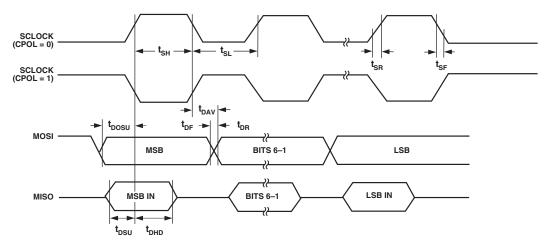
Figure 76. SPI Master Mode Timing (CPHA = 0)
