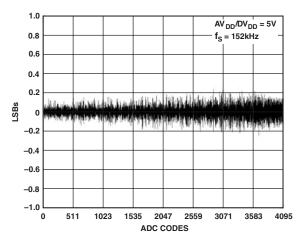
TPC 5. Typical DNL Error,  $V_{DD} = 5 V$
