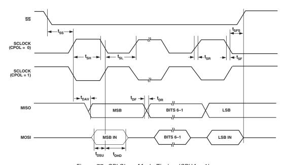
Figure 77. SPI Slave Mode Timing (CPHA = 1)
