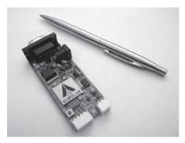
Figure 67. Accutron Single Pin Emulator
