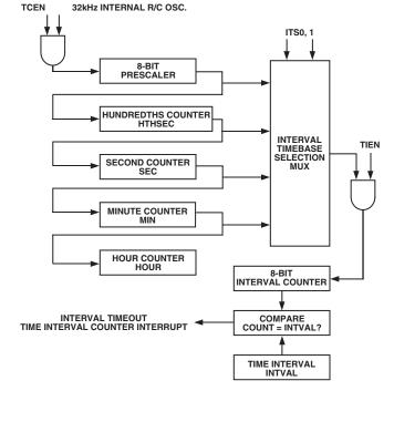
Figure 35. TIC, Simplified Block Diagram
