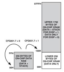
Figure 3. Extended Stack Pointer Operation
