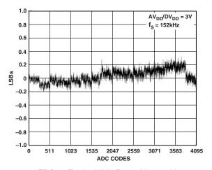
TPC 2. Typical INL Error,  $V_{DD} = 3 V$
