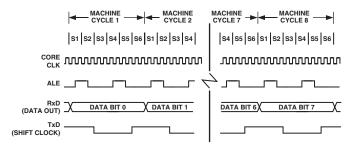
Figure 51. UART Serial Port Transmission, Mode 0
