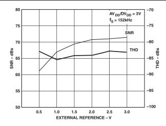
TPC 14. Typical Dynamic Performance vs.  $V_{REF}$ ,  $V_{DD} = 3 \text{ V}$
