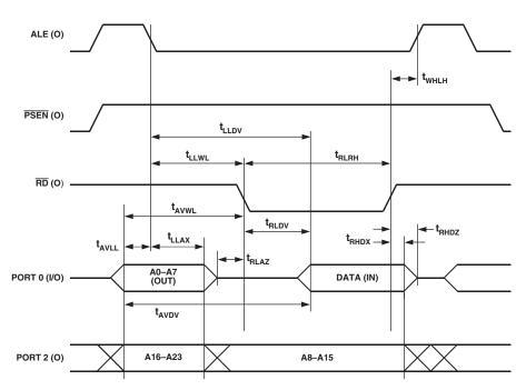
Figure 71. External Data Memory Read Cycle
