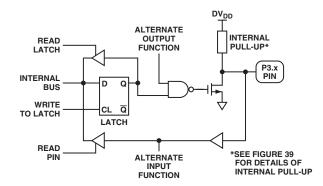
Figure 40. Port 3 Bit Latch and I/O Buffer
