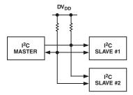
Figure 34. Typical I<sup>2</sup>C System
