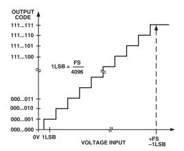
Figure 7. ADC Transfer Function
