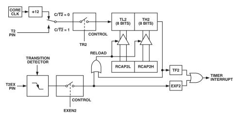
Figure 49. Timer/Counter 2, 16-Bit Autoreload Mode
