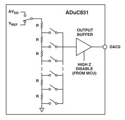
Figure 21. Resistor String DAC Functional Equivalent
