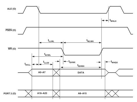
Figure 72. External Data Memory Write Cycle
