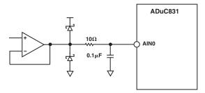
Figure 10. Buffering Analog Inputs
