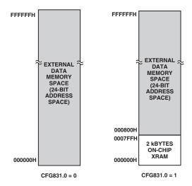
Figure 4. Internal and External XRAM
