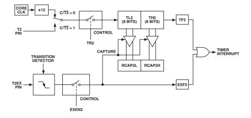
Figure 50. Timer/Counter 2, 16-Bit Capture Mode
