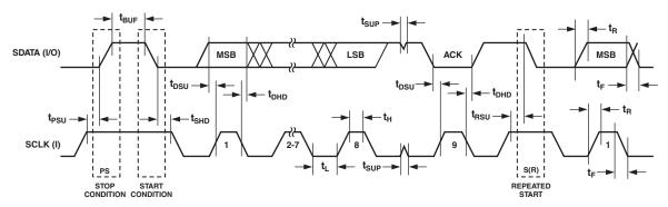
Figure 74. I<sup>2</sup>C Compatible Interface Timing
