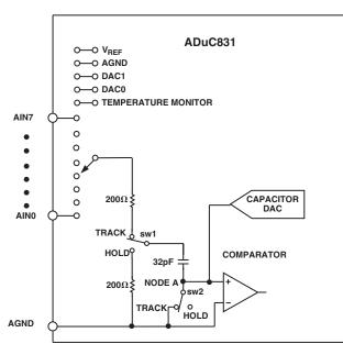
Figure 9. Internal ADC Structure
