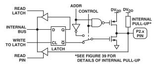
Figure 38. Port 2 Bit Latch and I/O Buffer
