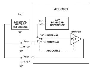
Figure 12. Using an External Voltage Reference
