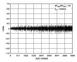
TPC 6. Typical DNL Error,  $V_{DD} = 3 V$
