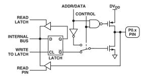
Figure 36. Port 0 Bit Latch and I/O Buffer
