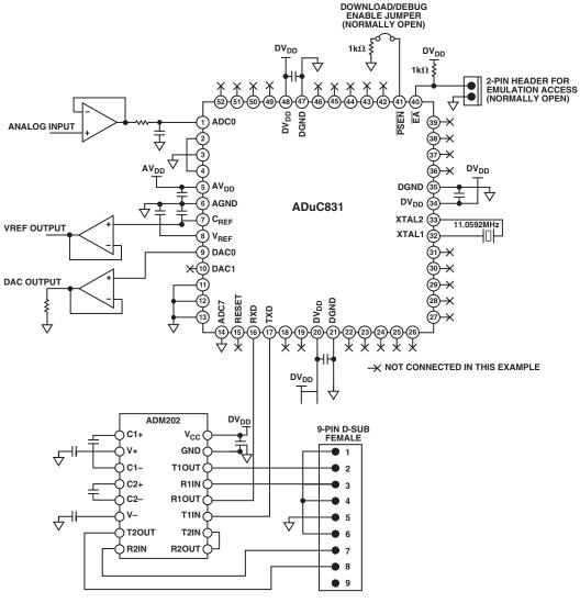
Figure 64. Example ADuC831 System (PQFP Package)
