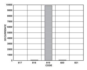
TPC 10. Code Histogram Plot,  $V_{DD} = 3 V$
