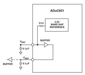
Figure 11. Decoupling  $V_{REF}$  and  $C_{REF}$
