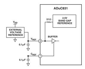
Figure 13. Using an External Voltage Reference
