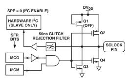
Figure 42. SCLOCK Pin I/O Functional Equivalent in I<sup>2</sup>C Mode
