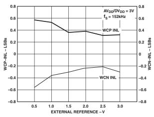
TPC 4. Typical Worst Case INL Error vs.  $V_{REF_r}$   $V_{DD} = 3 V$
