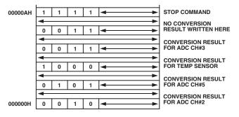
Figure 15. Typical External Memory Configuration Post ADC DMA Operation
