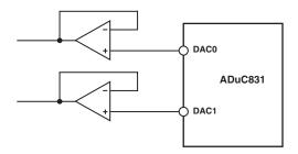
Figure 25. Buffering the DAC Outputs
