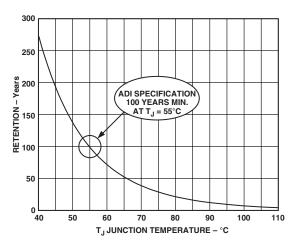
Figure 18. Flash/EE Memory Data Retention
