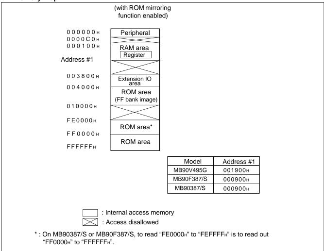
Note: When internal ROM is operating, F<sup>2</sup>MC-16LX allows viewing ROM data image on FF bank at upper-level of 00 bank. This function is called "mirroring ROM," which allows effective use of C compiler small model. F<sup>2</sup>MC-16LX assigns the same low order 16-bit address to FF bank and 00 bank, which allows referencing table in ROM without specifying "far" using pointer.
