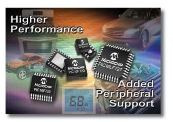
Mid-Range devices feature a 14-bit program word architecture and are available in 8 to 64-pin packages. These microcontrollers provide 1.8-5.5V operation, speeds up to 20 MHz, interrupt handling and an 8-level deep stack. These devices are available in various peripheral and memory configurations and feature serial analog and digital peripherals, such as: SPI, I<sup>2</sup>C, USART, LCD and A/D converters.
