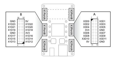
Each expansion header provides a bank of 12 I/O pins, which are mapped to the ports as described in the table on the next page.
