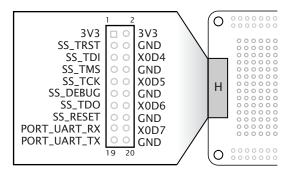
The XMOS XTAG connector converts between XSYS and USB 2.0, allowing the XC-2 to be connected to most PCs. On power on, the XS1-G4 boots from the on-board flash memory. The XS1-G4 can then be put into JTAG mode by the PC, which then boots another program.
