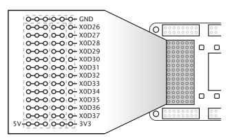
The prototyping area provides a bank of 12 I/O pins, which are mapped to the ports as described in the table below.
