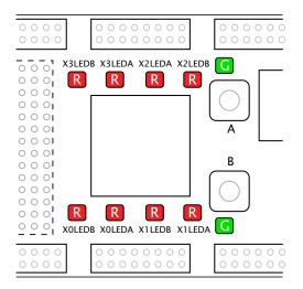
There are two green LEDs next to the two push-button switches and four red LEDs on both sides of the XS1-G4. Each LED is connected to a different pin, all of which are mapped to ports as described in the table below.
