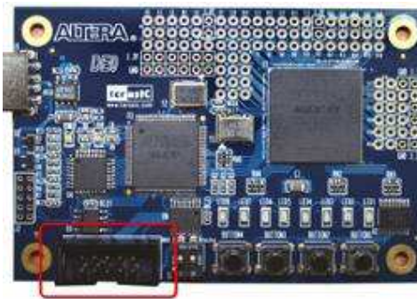
Figure 2.9. Solder a 10-pin header onto the MAX II Micro board
