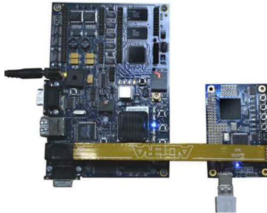
Figure 2.11. Use MAX II Micro as a USB Blaster cable and connect to another Altera board (NIOS II Kit in this case).
