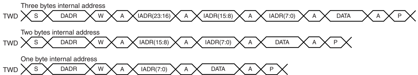
Figure 33-11. Master Write with One, Two or Three Bytes Internal Address and One Data Byte
