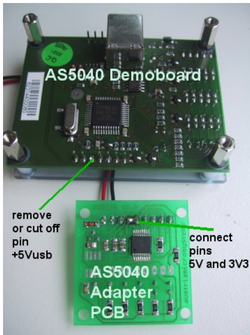
Figure 9: configuring the Adapter PCB for 3.3V operation
