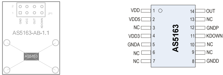
Figure 3: AS5163 adapter board connectors and encoder pinout
