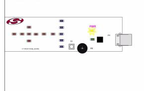
Move a hand in close proximity to the board. This causes the array of blue LEDs to light up as the hand approaches. Adjust proximity sensitivity by rotating the potentiometer R9.
