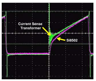
Figure 8. Leading-Edge Noise Suppression Waveforms (200 kHz, 9.3 A Load)
