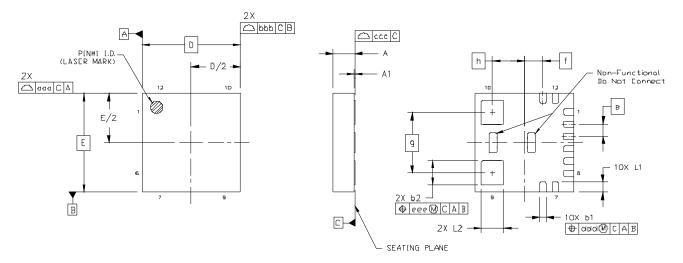
Figure 22. 12-Pin QFN Package Diagram
