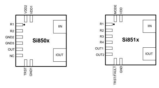
Figure 20. Example Pin Configurations
