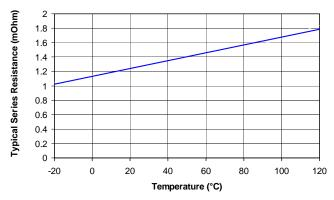
Figure 7. Series Resistance Thermal Characteristics
