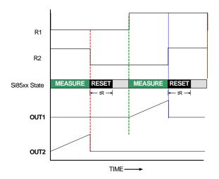
Figure 10. Two-Phase Buck Timing Example A
