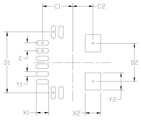
Figure 23. 12-Pin QFN PCB Land Pattern
