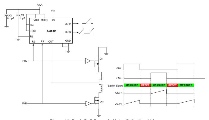
Figure 19. Push-Pull Example Using Default t<sub>R</sub> Value
