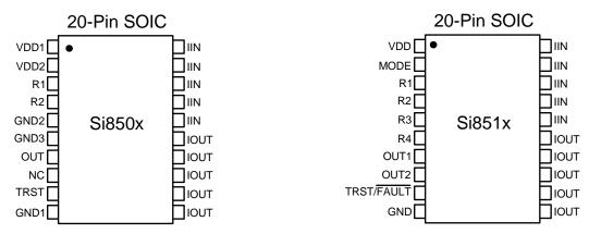
Figure 21. Example Pin Configurations
