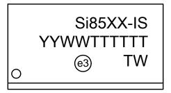
Figure 27. SOIC Top Marking
