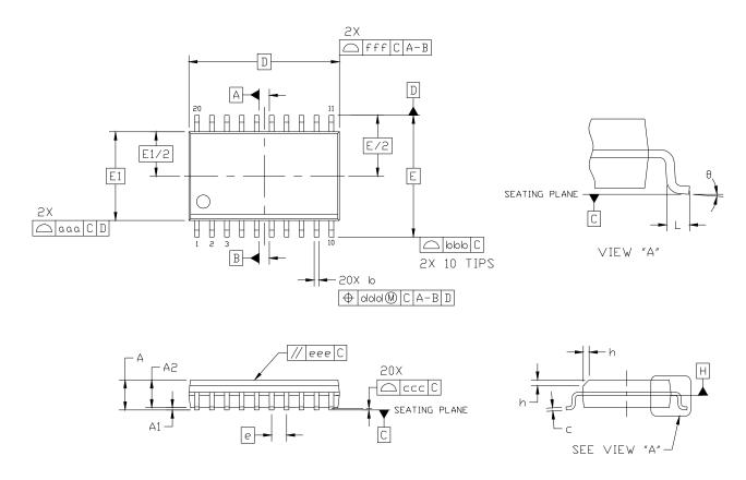
Figure 25. 20-Pin Wide Body SOIC
