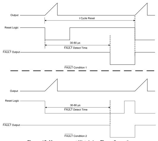
Figure 15. Measurement Watchdog Timer Operation
