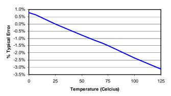
Figure 6. Differential Temperature Calibration Error
