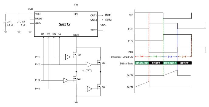
Figure 18. Full-Bridge Converter
