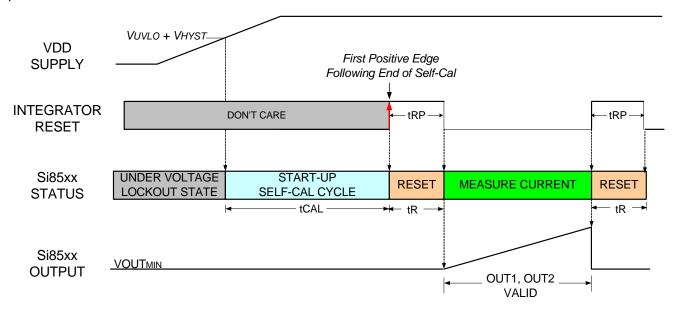
Figure 4. Si85xx Startup and Control Timing
