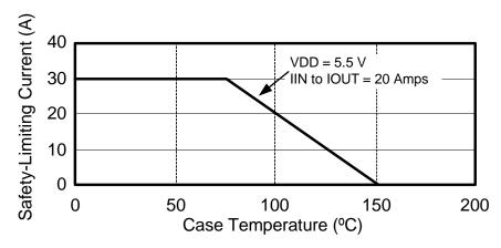
Figure 1. SOIC-20 Thermal Derating Curve, Dependence of Safety Limiting Values with Case Temperature per DIN EN 60747-5-2
