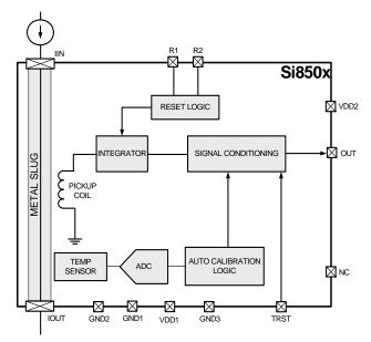
Figure 2. Si850x (Single Output) Block Diagram
