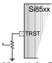
Figure 5. Programming Reset Time (t<sub>R</sub>)
