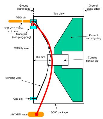
Figure 9. SOIC Layout Requirements
