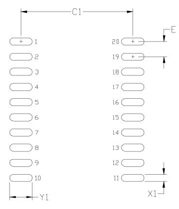
Figure 26. 20-Pin SOIC PCB Land Pattern
