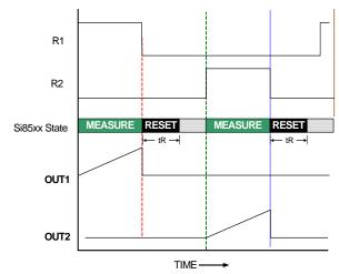
Figure 11. Full-Bridge Timing Example B
