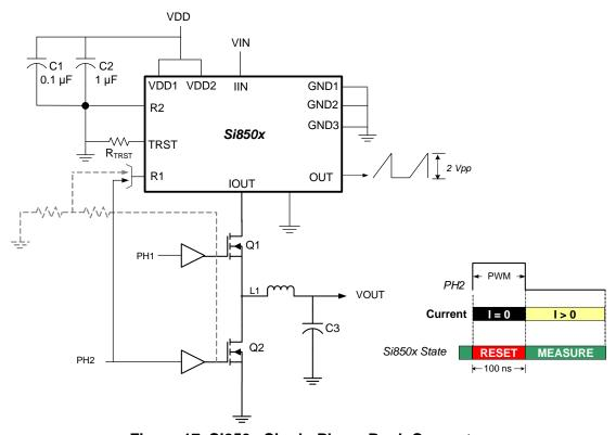
Figure 17. Si850x Single-Phase Buck Converter
