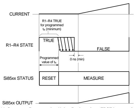
Figure 14. Correct t<sub>R</sub> Programming Using Resistor from TRST Input to Ground
