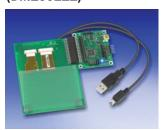
The mTouch Projected Capacitive Development Kit includes a 3.5" sensor mounted on a sensor board, a projected-capacitive board with the PIC16F707 MCU and fully functional firmware. The kit enables users to connect sensors to up to 24 channels without modifying the firmware.
