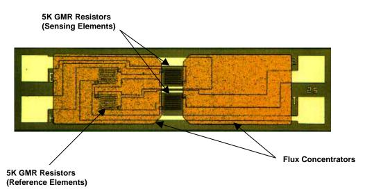
The size of this IC is approximately 350 microns by 1400 microns. The sensor is configured as a Wheatstone bridge. The serpentine structures in the center of the die and to the left of center under the large plated structure are 5 k $\Omega$  resistors made of GMR material.
