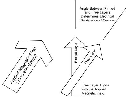
The percent change of resistance available with this GMR material is about 5%. The output is a cosine function over 360 degrees of angular movement by the external, saturating magnetic field.
