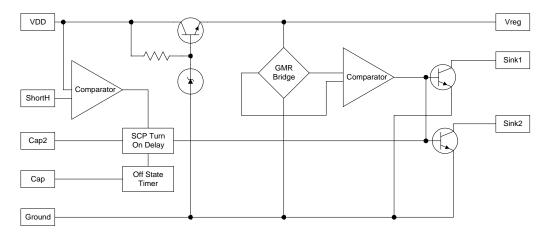
These digital sensors with SCP are available for use with current sinking or current sourcing outputs, in a range of magnetic field operate points. They are provided in an MSOP8 package with the cross-axis direction of sensitivity. An LED driver to indicate the presence of the magnetic field is also standard on these products. An SOIC8 package and standard axis sensitivity are available on a special order basis.
