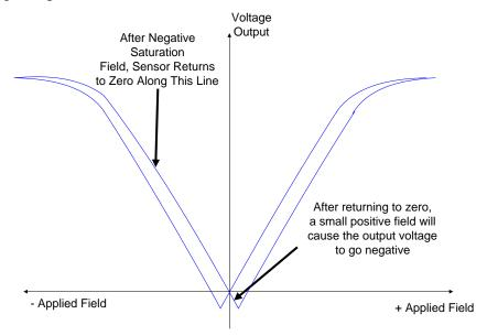
The same small positive field, applied after a positive saturating field, will result in a positive voltage output:
