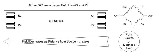
Note that if a uniform magnetic field is applied to the sensor IC, all the resistive sensor elements will change at the same time and the same amount, thus leading to no signal output from the bridge terminals. Therefore, a differential sensor cannot be used as a magnetometer or an absolute field detector; it must be used to detect the presence of a magnetic gradient field.
