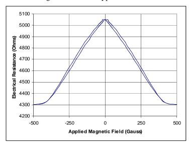
The following chart shows a typical characteristic for NVE's standard multilayer GMR material:
