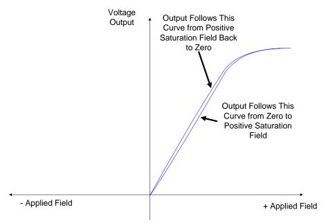
In the case of a unipolar field, the sensor is operating on the minor hysteresis loop. The hysteresis in this case is relatively small.
