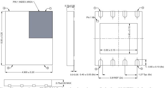
Note: Dimensions in mm. TDFN SO8 Package has thermal power dissipation of 240°C/Watt in free air. Attaching the package to a circuit board improves thermal performance.
