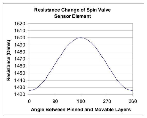
Four individual sensor resistors are supplied in the package, each with the pinned layer rotated 90° with respect to that of the previous sensor. These resistors can be connected in two half-bridge configurations to provide a sine and cosine output or monitored individually to provide an absolute indication of the angle between the pinned layer and the movable layer.
