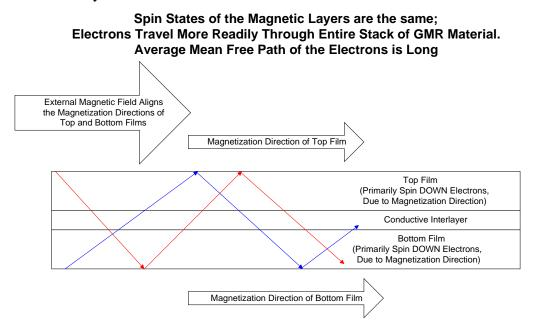
Note that the mean free path length of the electrons has now increased. This results in an overall lower electrical resistance for the GMR material. The change in resistivity of the material is shown on the path length diagram below:
