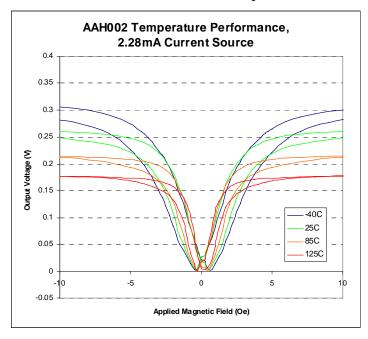
The next graph shows the temperature behavior of an AAL002-02 sensor, which is representative of the GMR material used in NVE's AAL, ABL, and AKL-Series products:
