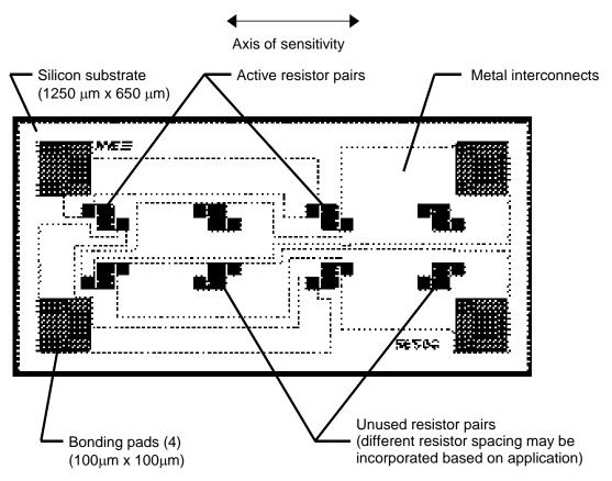
BASIC GRADIOMETER BRIDGE SENSOR LAYOUT
