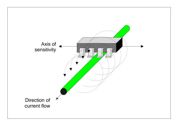
SENSING MAGNETIC FIELD FROM A CURRENT-CARRYING WIRE
