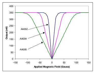
Maximum signal output from such a sensor element is typically 350 mV at 100 Gauss with a 5V power supply. This compares to an output of 5 mV under the same conditions for a Hall sensor element, and 100 mV for an AMR sensor.
