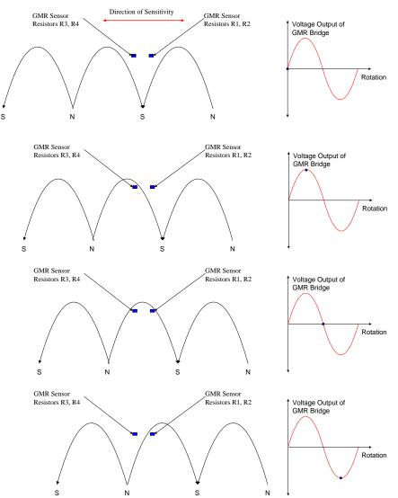
Note that in this case, as long as the sensor is positioned symmetrically with the encoder, offset is minimized. Also note that the GT Sensor provides one full sine wave output for each magnetic pole. This is double the frequency of a Hall effect sensor, which provides one full sine wave output for each north-south pole pair. As a result, replacing a Hall sensor with a GT sensor doubles the resolution of the output signal.
