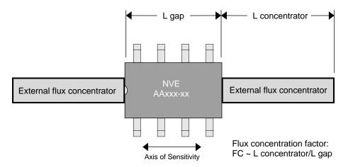
Elongated pieces of soft magnetic material gather external magnetic flux and expose the sensor to a magnetic field that is larger than the external magnetic field. For best results, two pieces of soft magnetic material of the same size are used. The concentration factor is approximately the ratio of one
