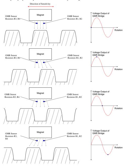
Despite the simplicity of the preceding drawings, magnetically biasing a gear tooth for a production product can be complex. Typically, the position of the sensor relative to the magnet is fixed, but there is a variation in the airgap between the sensor and the target gear tooth. This can lead to magnetic conditions that can cause an unstable output.
