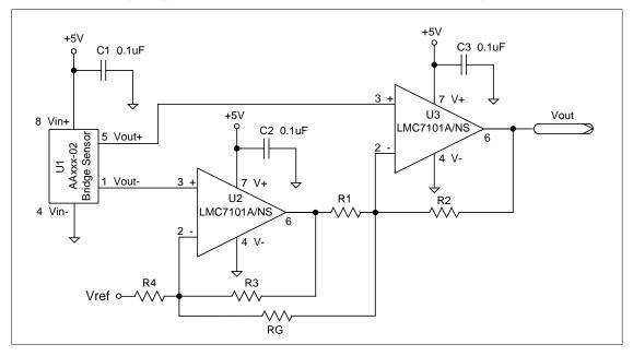
Two Op Amp Preamplifier Circuit
