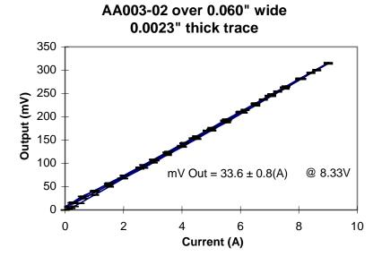
The current in this trace was swept from zero to nine Amps, similarly to the 90-mil analysis. The sensor output to current correlation from this graph is  $4.0 \pm 0.1 \text{ mV/V/A}$ . The differences between the 90 and 60-mil traces is due to the field distribution/density differences between the two due to the difference in width.
