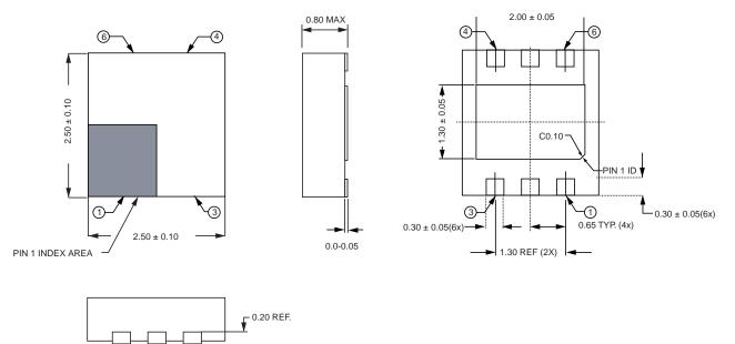
Note: Dimensions in mm. TDFN6 package has thermal power dissipation of 320°C/Watt in free air. Attaching the package to a circuit board improves thermal performance.
