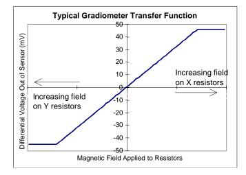
GRADIOMETER BRIDGE SENSOR OUTPUT CHARACTERISTIC
