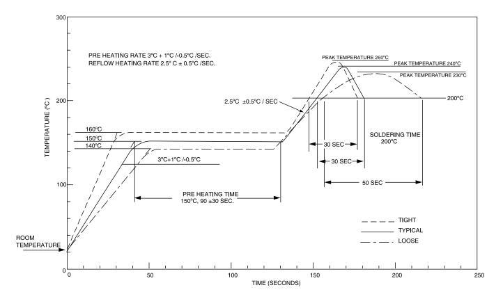
For leaded (Pb) parts, the peak temperature shown in this profile can be decreased to as low as 230°C.
