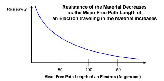
In order to take advantage of this effect, GMR films are manufactured with very thin layers of alternating magnetic and non-magnetic materials. This is done to allow magnetic modulation of the electron spin in the materials. The spin dependence of conduction electrons in magnetic materials, along with the increasing resistivity at very small material thicknesses, combine to make the GMR effect possible.
