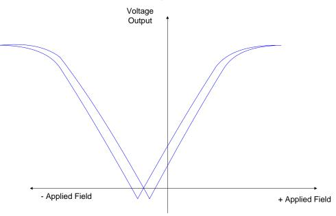
With this approach, a small applied field to the sensor will result in a bipolar output signal. Furthermore, the slope of the signal characteristic will be the same no matter which curve the sensor is operating on. So, the magnetic sensitivity of the device is the same, no matter how much hysteresis the sensor has.
