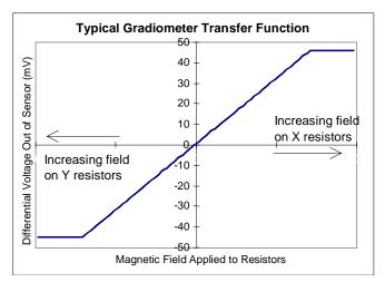
The Figure at left is a simulated output from an NVE Gradiometer. The output / gradient correlation shown assumes one pair of resistors is held at zero field. Note the bipolar output.
