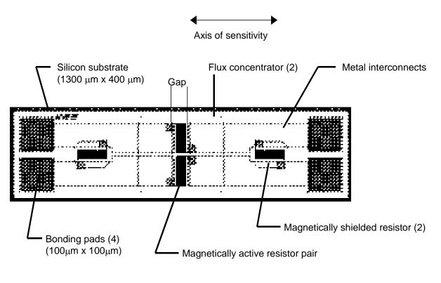
TYPICAL GMR MAGNETIC FIELD SENSOR LAYOUT
