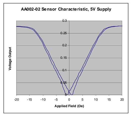
GMR MAGNETIC FIELD SENSOR OUTPUT CHARACTERISTIC
