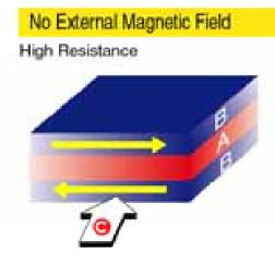
Is a conductive, nonmagnetic interlayer. Magnetic moments in alloy (i) layers face opposite directions due to the anti-ferromagnetic coupling. Resistance to current (is high.)
