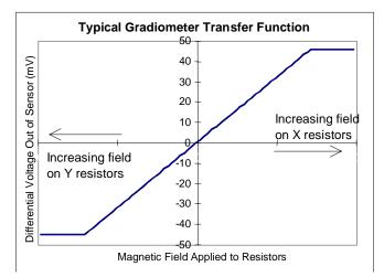
The Figure at left is a simulated output from an NVE Gradiometer. The output / gradient correlation shown assumes one pair of resistors is held at zero field. Note the bipolar output.
