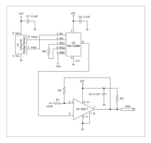
THRESHOLD DETECTION CIRCUIT
