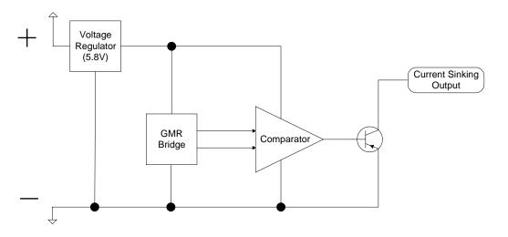
The GMR Switch holds its precise magnetic operate point over extreme variations in temperature and power supply voltage. This low cost product has revolutionized the industrial control position sensing market.
