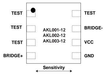
Note: Bridge + and Bridge - are provided for analysis purposes only. NVE does not recommend connecting these pins in a production product for ESD and loading reasons. Also, all pins labeled "Test" must be floating, *i.e.*, not connected to each other or any other circuit node.
