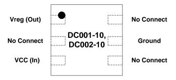
Note: The die attach pad is exposed on the back of this package. NVE recommends that it be connected to the ground pin and the PCB for improved temperature performance.
