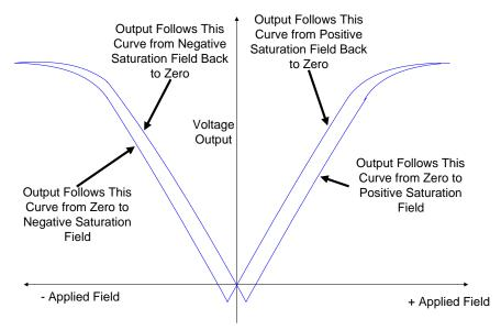
In this case the sensor is operating on the major hysteresis loop, so the hysteresis shown by the output characteristic of the sensor is relatively large. This is the worst-case hysteresis exhibited by the sensor element.
