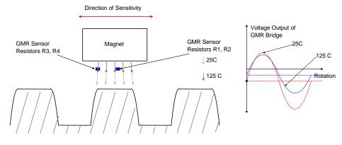
Finally, as the airgap changes, the magnetic field at the sensor also changes. So, the magnetic field at the sensor will vary from one installation to the next, and if the gear has runout, wobble, or expands with temperature, the output signal and offset of the sensor element will vary.
