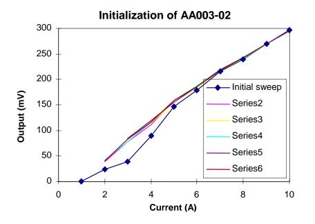
The initial sweep data has deviated from the other series of current sweeps. After the first sweep was completed, the subsequent five sweeps fell right on each other. This shows that a lower error can be obtained by "initializing" the sensor. After initialization, the error will be much lower until the working current range is exceeded in either direction. Saturation of the device (currents in the 20A range) as well as changing the applied current direction will increase the hysteresis/error.
