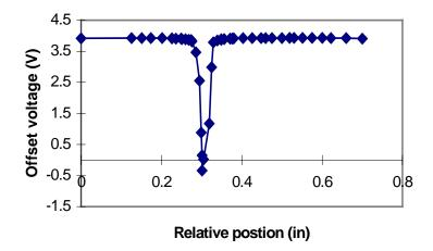
The graph below shows the variation in signal at the sensor as the currency is moved farther away from the GMR sensor element. Close proximity to the sensor is important in order to maximize output signal from the sensor.
