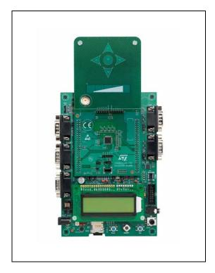
The kit contains an STM8/128-EVAL board, and an STM8S touch sensing evaluation daughterboard (STM8Sxxx-TS1) which provides an evaluation platform for the resistor-capacitor acquisition principle.
