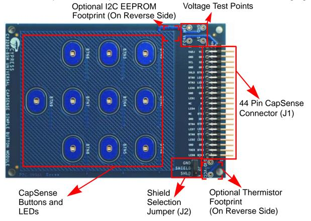
The module consist of ten CapSense buttons and ten LEDs. These are interfaced to the CapSense controller board via 44 pin receptacle connector (J1). A three pin jumper (J2) is provided for selection between shield electrode and ground. The board also incorporates an optional I2C EEPROM and thermistor that are not populated by default.
