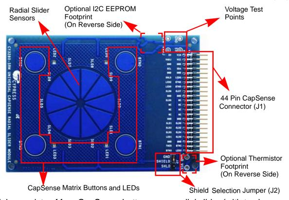
The module consists of four CapSense buttons, one radial slider (with twelve sensors), and four LEDs. These are interfaced to the CapSense controller board via 44 pin receptacle connector (J1). A three pin jumper (J2) is provided for selection between shield electrode and ground. The board also incorporates an optional I2C EEPROM and thermistor that are not populated by default.
