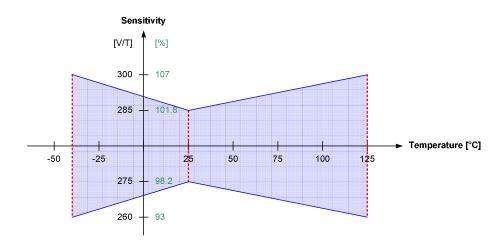
The corresponding sensitivity performance for the high field version is  $100V/T \pm 1.5 V/T$  at room temperature and  $100V/T \pm 7 V/T$  over the temperature range from -40 to 125 °C.
