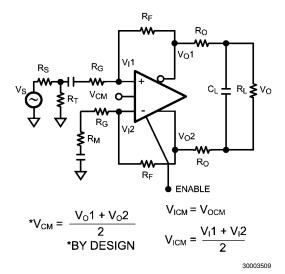
FIGURE 5. AC Coupled for Single Supply Operation
