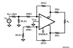
FIGURE 4. Single Ended Input S-Parameter Test Circuit  $(50\Omega \text{ System})$
