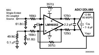
FIGURE 7. Driving a 12-bit ADC
