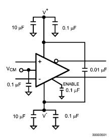
FIGURE 12. Split Supply Bypassing Capacitors
