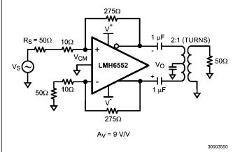
**FIGURE 6. Noise Figure Circuit Configuration**
