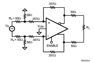
FIGURE 2. Differential S-Parameter Test Circuit
