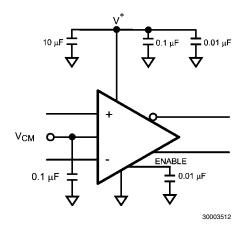
FIGURE 13. Single Supply Bypassing Capacitors
