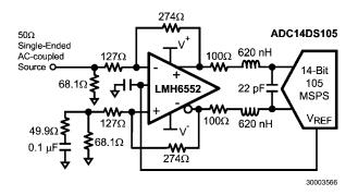
FIGURE 9. Driving a 14-bit ADC
