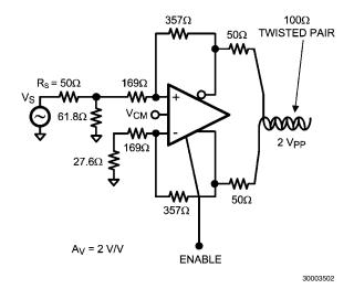
FIGURE 11. Fully Differential Cable Driver
