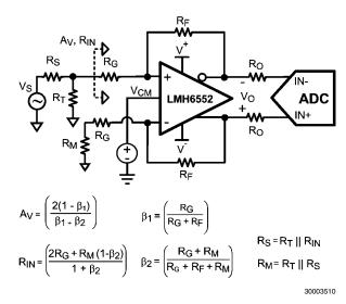
FIGURE 3. Single Ended Input with Differential Output
