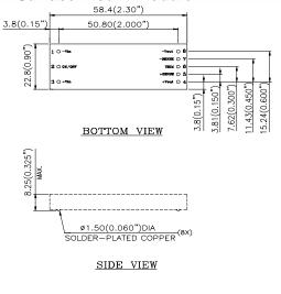
NOTES: DIMENSIONS ARE IN MILLIMETERS AND (INCHES) TOLERANCES: X.Xmm±0.5mm(X.XX in.±0.02 in.) X.XXmm±0.25mm(X.XXX in.±0.010 in.)
