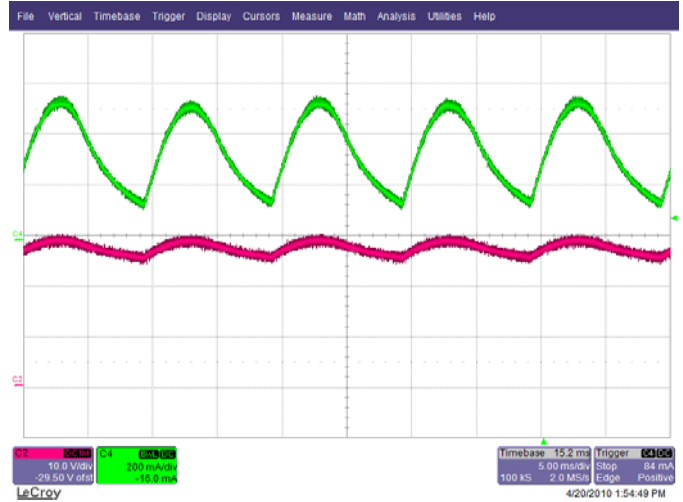
Figure 22 – 265 VAC, Full Load. Upper: I_{RIPPLE} , 0.2 A / div. Lower: V_{OUTPUT} 10 V, 5 ms / div.
