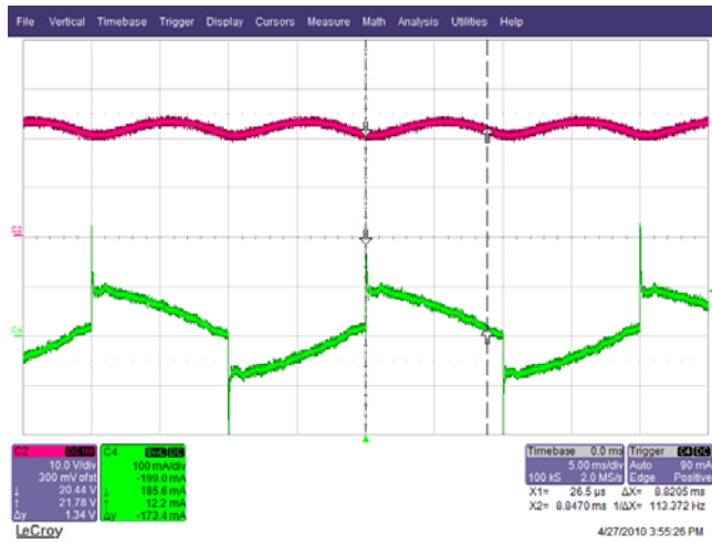
Figure 34 – 230 VAC, Full Phase. Upper: V OUT , 10 V / div. Lower: I IN , 0.1 A / div., 5 ms / div.
