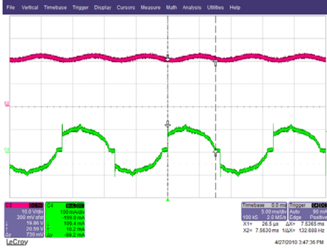
Figure 30 – 115 VAC, Full Phase. Upper: V_{OUT} , 10 V / div. Lower: I_{IN} , 0.1 A / div., 5 ms / div.
