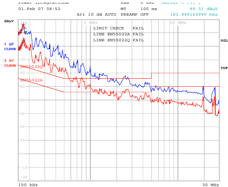
Figure 21 – Conducted EMI at 115VAC of competitive product.
