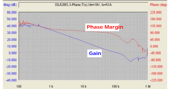
FIGURE 53. REFERENCE DESIGN LOOP GAIN T2(s) MEASUREMENT RESULT
