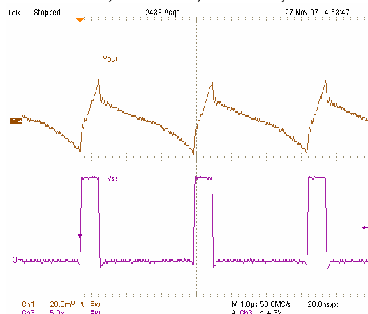
Fig. 6 Output Voltage Ripple at 25A Load
