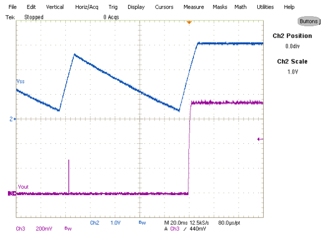
Fig. 12: Short (Hiccup) Recovery, V_p: 0.6V Ch_2: V_{ss} , Ch_3: V_{out}
