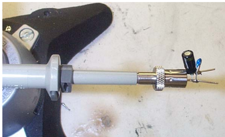
Figure 30 – Oscilloscope Probe with Probe Master 5125BA BNC Adapter. (Modified with wires for probe ground for ripple measurement, and two parallel decoupling capacitors added).
