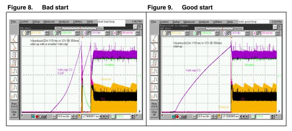
In *Figure 8* the purple trace is the V<sub>dd</sub> voltage rising to ~14 V. The energy with the 2.2  $\mu$ F capacitor does not store enough energy. As seen the output voltage (green trace) does not reach high enough to bootstrap, It succeeds the second time after there is a partial charge on the output cap. *Figure 9* is using a 4.7  $\mu$ F V<sub>dd</sub> cap. With adequate energy the power supply starts the first time.
