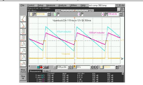
Figure 2. Inductor current: 470 µH VS 1000 µH
