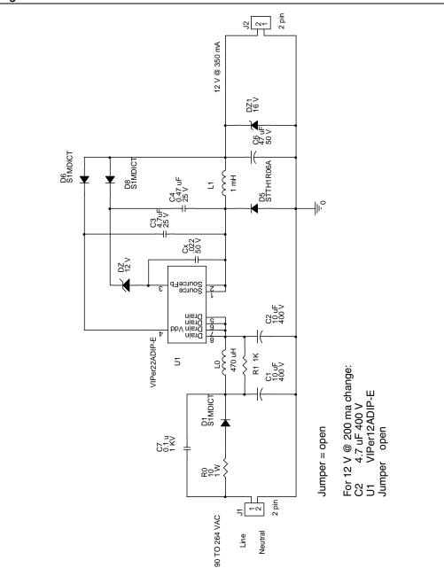
Figure 3. Schematic for 12 V at 350 mA
