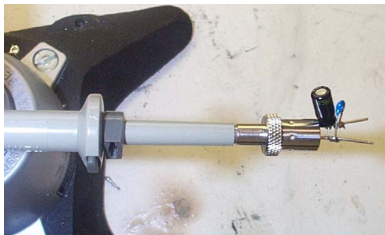
Figure 23 – Oscilloscope Probe with Probe Master 5125BA BNC Adapter (Modified with wires for probe ground for ripple measurement, and two parallel decoupling capacitors added).
