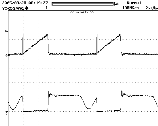
Figure 12 – 90 VAC, Full Load. Upper: I_{DRAIN} , 0.10 A / div. Lower: V_{DRAIN} , 200 V, 2 \mu s / div.
