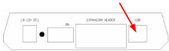
Figure 5. ADC08(D)XXXXDEV rear panel showing location of USB connector
