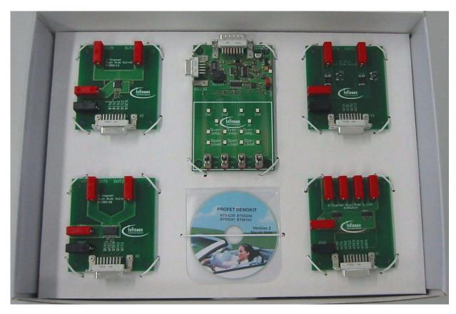
The PROFET Demo Kit consists of five different boards devided in two types. The PROFET are mounted on the power boards which also contain 4 mm plug sockets for power supply and loads. The power boards are connected via a D-SUB-15 connector to the control board. The complete PROFET Demo Kit is reverse polarity protected.
