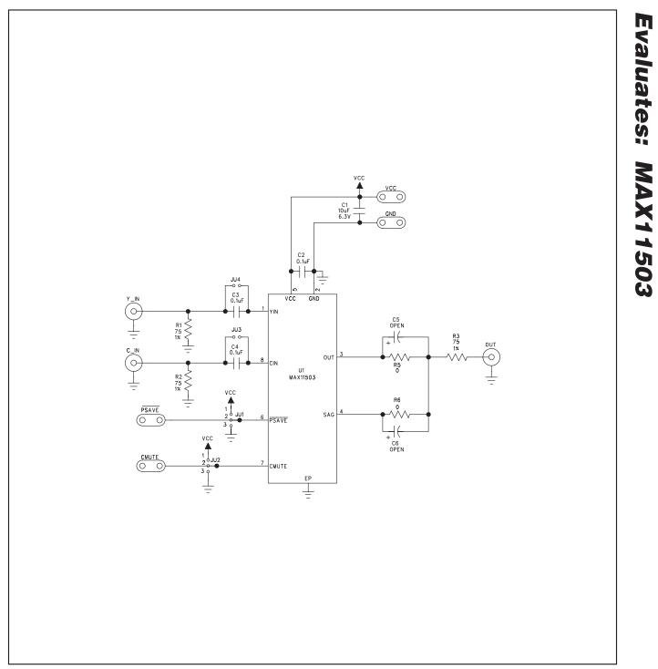
Figure 1. MAX11503 EV Kit Schematic
