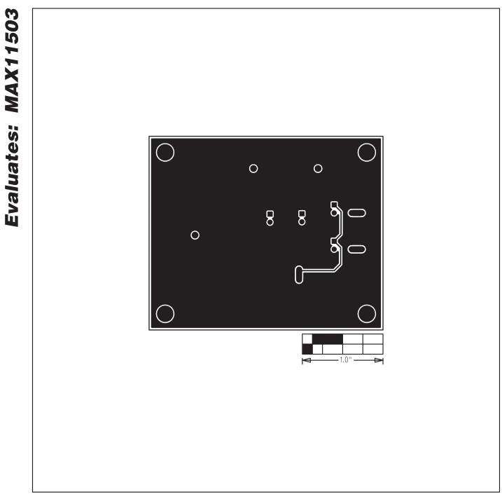
Figure 4. MAX11503 EV Kit PCB Layout—Solder Side
