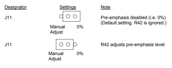
When the jumper J11 is set to MANUAL ADJUST, a 2K-Ohm potentiometer (R42) can be adjusted using a jeweler's screwdriver to increase or decrease preemphasis. Turning clockwise increases pre-emphasis; turning counterclockwise decreases pre-emphasis.
