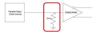
On-board transmitter LVCMOS/LVTTL input termination resistors (R1 – R25)
