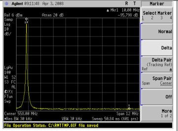
Spur at 10 MHz offset for a frequency of 553 MHz is below the spectrum analyzer noise floor.
