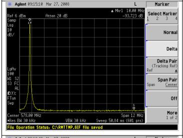
Spur at 10 MHz offset for a frequency of 573 MHz is below the spectrum analyzer noise floor.
