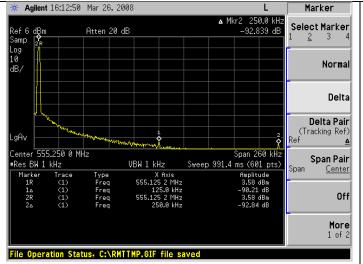
Spur at 250 kHz offset at a frequency of 555.125 MHz is –92.5 dBc. Since this mode uses the divide by 2 mode, the channel spacing here is actually 125 kHz. The spur at 125 kHz could be completely eliminated changing the fractional denominator.
