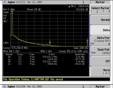
Spur at 250 kHz offset for a frequency of 575.125 MHz is -83.4 dBc.
