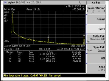
Fractional Spur at 250 kHz offset at a worst case frequency of 1150.25 MHz is –73.3 dBc. The sub-fractional spur at 125 kHz offset of -81.3 dBc is also visible
