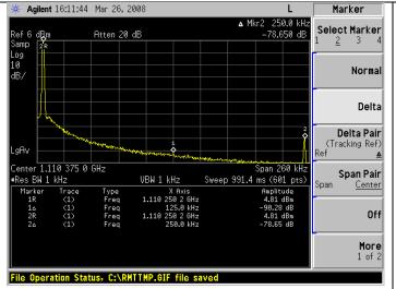
Fractional Spur at 250 kHz offset at a worst case frequency of 1110.25 MHz is –78.6 dBc. Worst case channels occur at exactly one channel spacing above or below a multiple of the crystal frequency.
