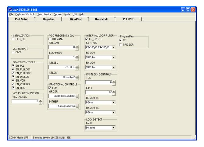
The Bits/Pins tab displays many of the bits used to program the part. Right mouse click any bit to view more information about what this does.
