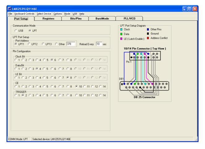
The port setup tells CodeLoader what information goes where. If this is wrong, the part will not program. Although LPT1 is usually correct, CodeLoader does NOT automatically detect the correct port. On some laptops, it may be LPT3.
