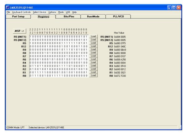
The Registers tab shows the literal bits that are being sent to the part. These are the registers every time the PLL is loaded by using the menu command or Ctrl+L. R5 (INIT1) and R5 (INIT 2) are just the R5 register being used to properly initialize the part. So a single CNT+L will load the part.
