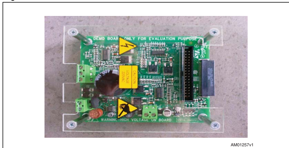
Figure 1. STEVAL-IHM021V1 demonstration board
