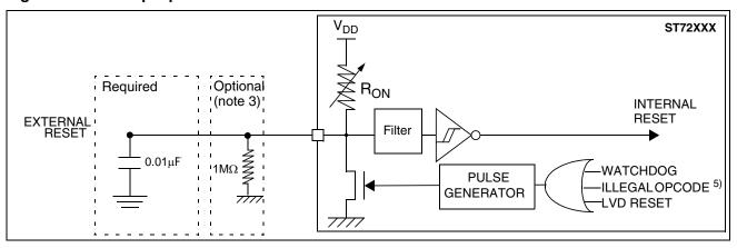
Figure 92. RESET pin protection when LVD is disabled. 1)
