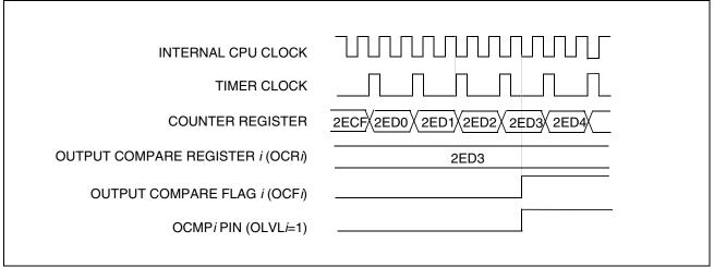
Figure 43. Output Compare Timing Diagram, f<sub>TIMER</sub> =f<sub>CPU</sub>/4
