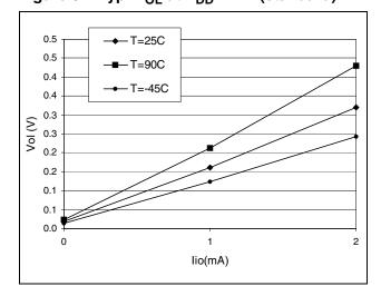
Figure 83. Typ. V<sub>OL</sub> at V<sub>DD</sub>=5V (high-sink)
