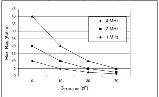
Figure 98. Recommended C<sub>AIN</sub>/R<sub>AIN</sub> values<sup>3)</sup>
