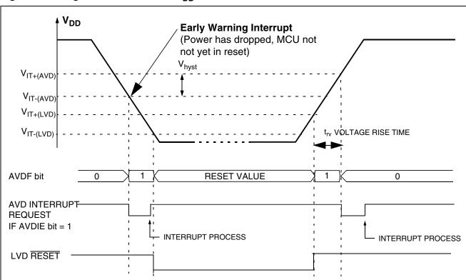
Figure 15. Using the AVD to Monitor V<sub>DD</sub>
