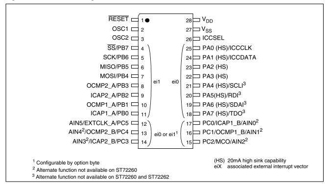
Figure 3. 32-Pin SDIP Package Pinout
