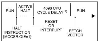
Figure 24. ACTIVE-HALT Mode Flowchart
