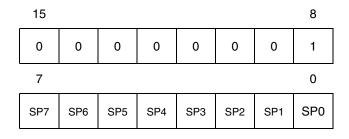
The Stack Pointer is a 16-bit register which is always pointing to the next free location in the stack. It is then decremented after data has been pushed onto the stack and incremented before data is popped from the stack (see Figure 8).
