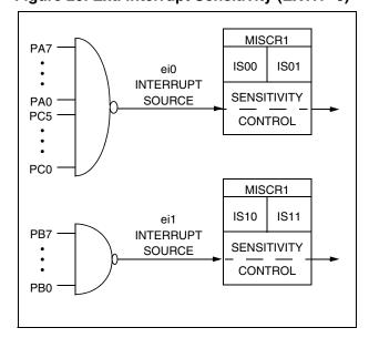
Figure 30. Ext. Interrupt Sensitivity (EXTIT=1)
