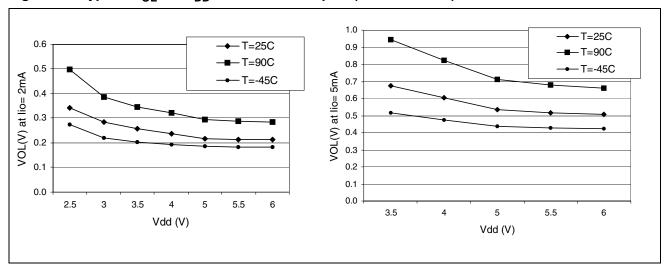
Figure 89. Typical V<sub>OL</sub> vs. V<sub>DD</sub> on high sink I/O port (Port A)
