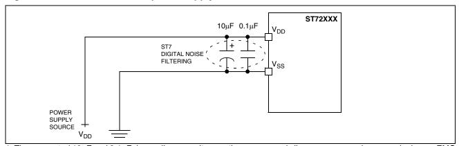
1. The suggested  $10\mu$ F and  $0.1\mu$ F decoupling capacitors on the power supply lines are proposed as a good price vs. EMC performance tradeoff. They have to be put as close as possible to the device power supply pins. Other EMC recommendations are given in AN1709.
