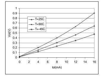
Figure 82. Typ. V<sub>OL</sub> at V<sub>DD</sub>=2.7V (standard)
