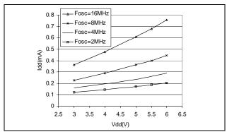
Figure 68. Typical I<sub>DD</sub> in WAIT at T<sub>A</sub>=25°C
