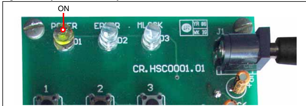
Figure 10. System stable, ready to use
