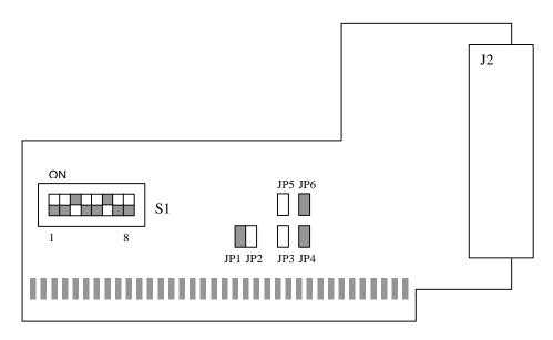
Switch S1 sets the base I/O address for the D12 evaluation board. Default base address is 0x368. The D12 evaluation board occupies 8 I/O locations. A0 to A2 are decoded on the D12 evaluation board. Switch S1 sets the address decoding of A3 to A9. Please notice that a switch 'ON' is logic '0'.
