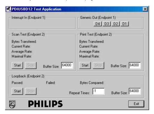
The operation of each endpoint is designed according to its nature that is supported in PDIUSBD12. Generic in and generic out endpoints has max packet size of 16 bytes and supports I/O access only. So they are suitable for small size and low rate data transfer like keyboard and logic controls. The main endpoints have max packet size of 64 bytes or 128 bytes with double buffering and DMA support. So they are suitable for high data rate, large size data transfer.
