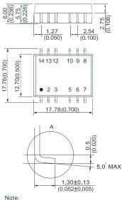
Unit:mm(inch) Pin section:0.60\*0.25mm(0.024\*0.010inch) Pin tolerances:±0.10mm(±0.004inch) General tolerances:±0.25mm(±0.010inch)
