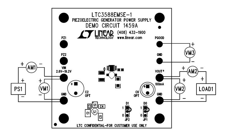
Figure 1. Proper Measurement Equipment Setup
