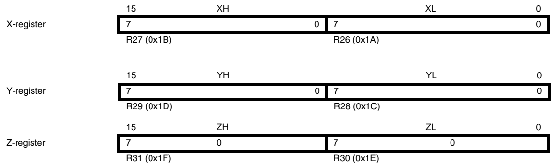
Figure 7-3. The X-, Y-, and Z-registers
