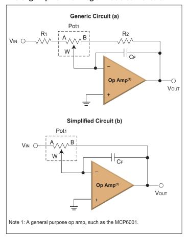
Equation 1-1 shows how to calcultate the gain for the simplified circuit (Figure 1-1b). The gain is the ratio of the digital potentiometers wiper position on the RAB resistor ladder. As the wiper moves away from the midscale value, the gain will either become greater then one (as wiper moves towards Terminal A), or less then one (as wiper moves towards Terminal B).
