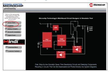
The Mindi Amplifier Designer & Simulator is an Application Circuit that generates full schematic diagrams of an amplifier circuit with recommended component values and displays the signal responses in frequency and time domains.
