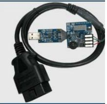
OBD-II standard SAE J1979. These modes allow the OBD Reader to access the current c show freeze frame data, and show the stored diagnostic trouble codes. The purpose of the reference design is to demonstrate an automotive Silicon Labs MCU interfacing to a vehic with a very simple and straightforward design. The MCU communicates with the vehicle u the CAN bus at 500 kbps and does not require an external crystal.
