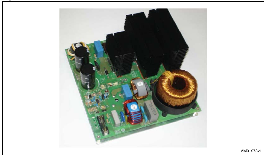
Figure 3. STEVAL-ISF001V1 demonstration board
