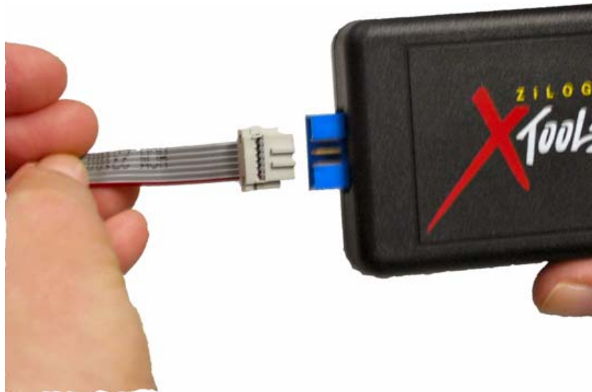
Figure 3. Connecting the Six-Conductor Ribbon Cable to the USB Smart Cable
